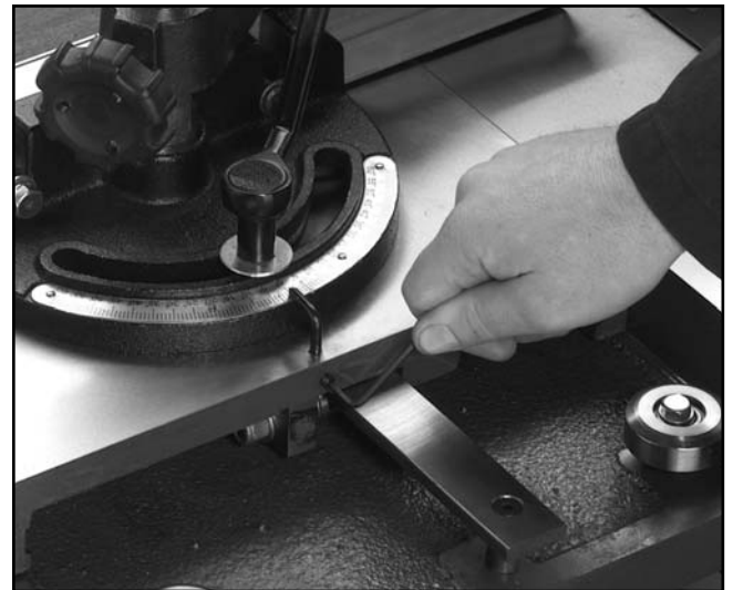
Figure 29. Setting the miter gauge pointer.
